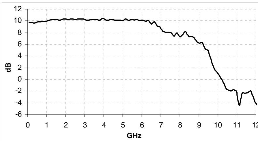
Figure 3: Frequency response of AMT8650-T46L-EVA (-20dBm optical input)
