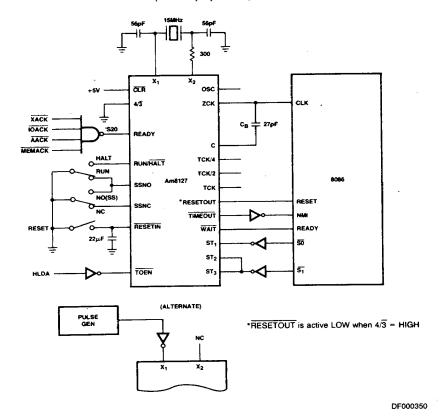
The typical operating configuration for Am8127 is shown above. The component values shown provide a 4MHz clock output for the AmZ8002 CPU. The 27pF capacitor from C to ZCK is a bootstrap to ensure clock rise to  $V_{\rm CC}$  -0.4V within
