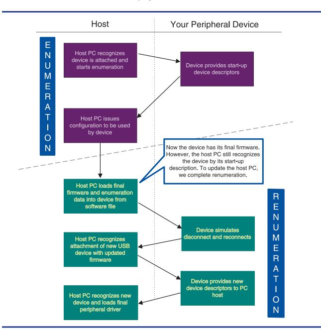
A USB hardware connection is simpler than current interface standards (ISA. PCI, serial, parallel, and SCSI). For example, there are no IRQs or DMAs to set. USB does not use direct connections like RS232 or **EPP** (Enhanced Parallel Port). Instead, USB is a packetized protocol similar to telecommunication standards such as X.25 or frame relay. This makes software development complex.
