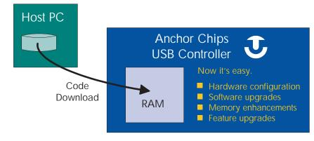
The focus of the EZ-USB family is to provide the peripheral designer a multitude of design configurations and migration paths. The "soft," programmable nature of the EZ-USB architecture provides flexibility while minimizing risks.
