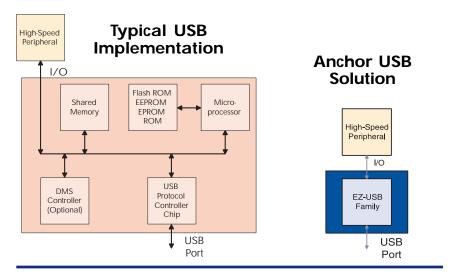
Anchor Chips' EZ-USB family eliminates the need to become an expert in USB. It allows the designer to take advantage of the benefits of USB without investing large amounts of time and energy. With the EZ-USB family, peripheral designers can have USB traffic running within hours, instead of weeks as with other USB solutions.
