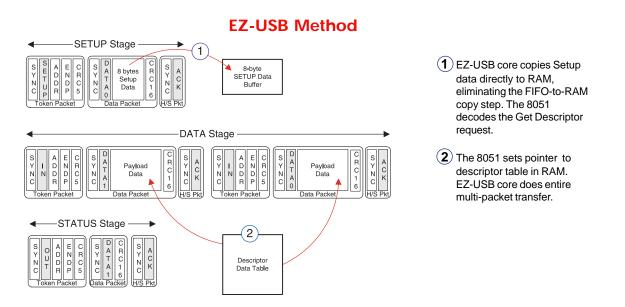
The EZ-USB core directly transfers setup packet data into a dedicated eight-byte Setup data buffer for CPU inspection (1). Then the 8051 loads an EZ-USB pointer with the start address of the requested descriptor data (2). The EZ-USB core does the rest. The EZ-USB core automatically takes care of error checking and retries, dividing the table into packets for the various IN transfers and responding to the Status stage.
