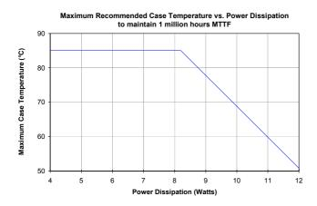
To calculate the MTTF for the module, the junction temperature needs to be determined. This can be easily calculated with the module's power dissipation, the thermal resistance value, and the case temperature of operation:
