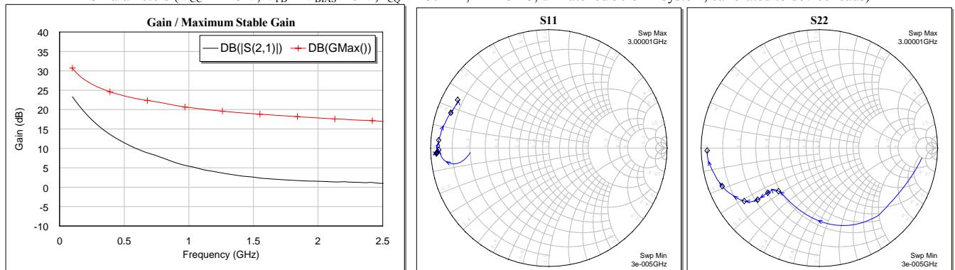
The gain for the unmatched device in 50 ohm system is shown as the trace in black color. For a tuned circuit for a particular frequency, it is expected that actual gain will be higher, up to the maximum stable gain. The maximum stable gain is shown in the marked red line. The impedance plots are shown from 50 – 3000 MHz, with markers placed at 0.5 – 3.0 GHz in 0.5 GHz increments.
