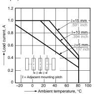
4.-(2) Load current vs. ambient temperature characteristics for adjacent mounting (DC output)
