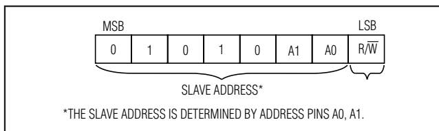
Figure 1. DS3502 Slave Address Byte
