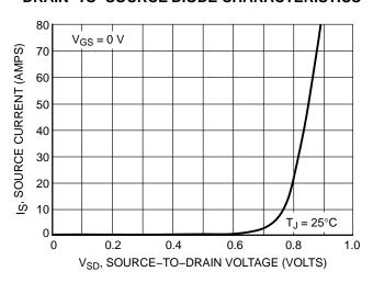
Figure 10. Diode Forward Voltage versus Current
