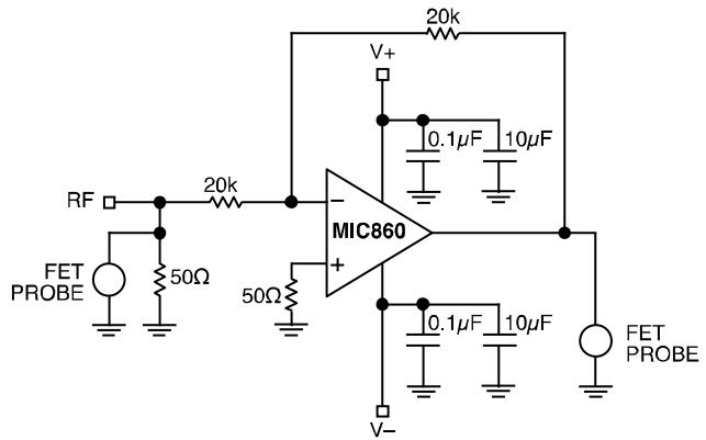
Test Circuit 4.  $A_V = -1$
