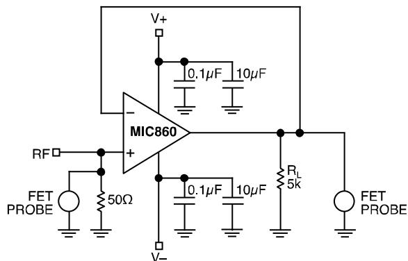
Test Circuit 3.  $A_V = 1$
