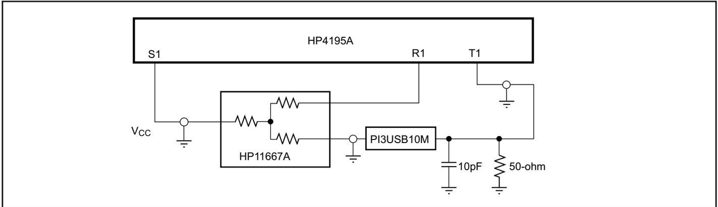
**Test Circuit for Electrical Characteristics**
