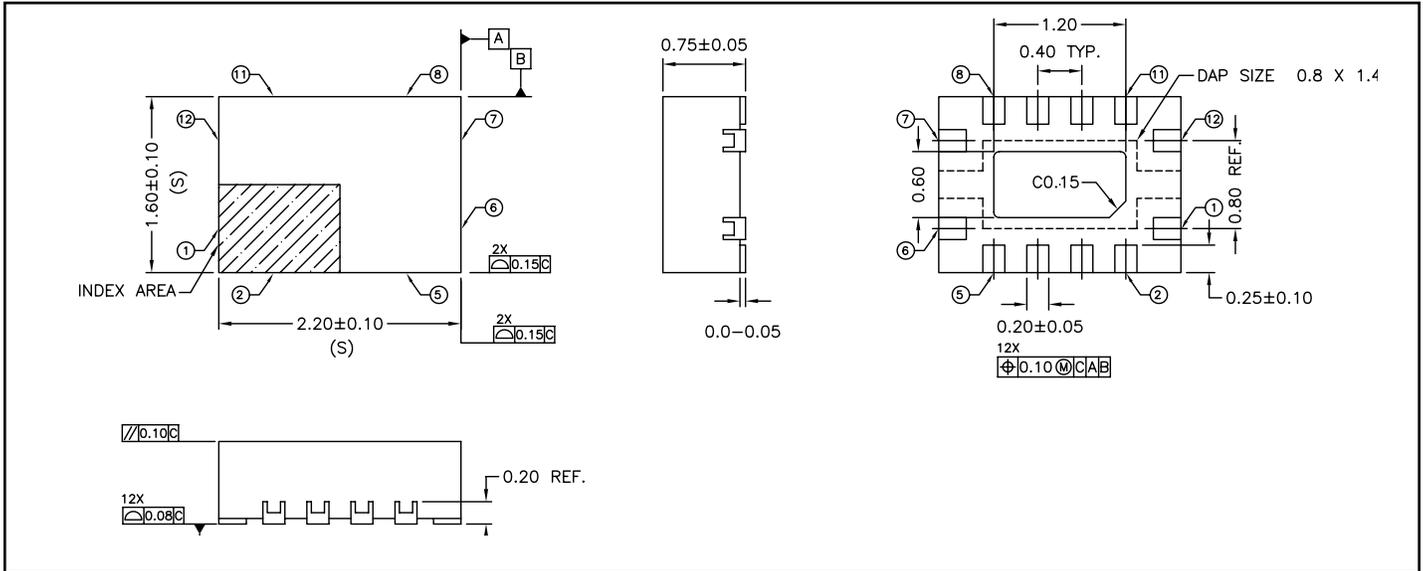
**Package Mechanical: 12-Contact TDFN (ZE)**
