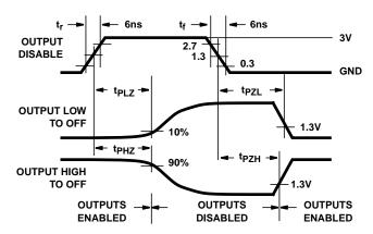
FIGURE 7. HC THREE-STATE PROPAGATION DELAY WAVEFORM
