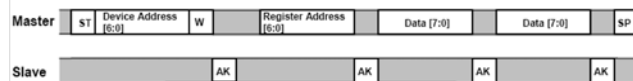
Figure 10. Multiple Byte Writes - The Master (MCU) is writing to multiple sequential registers of the MMA7450L
