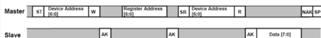
Figure 7. Single Byte Read - The Master is reading one address from the MMA7450L
