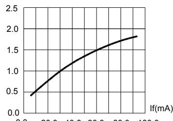
FIG.3 RELATIVE LUMINOUS FLUX VS.
