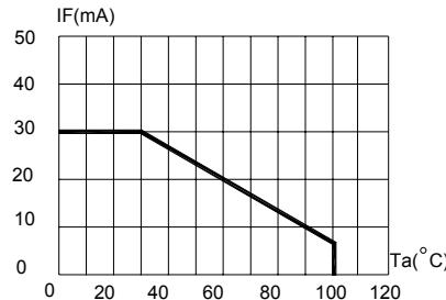
FIG.5 MAXIMUM FORWARD DC CURRENT VS
