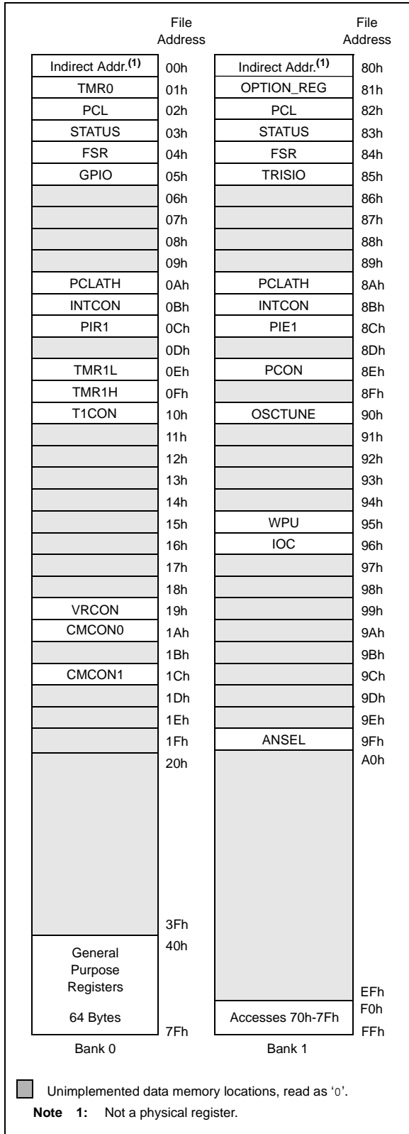
FIGURE 2-2: DATA MEMORY MAP OF THE PIC12F609/HV609
