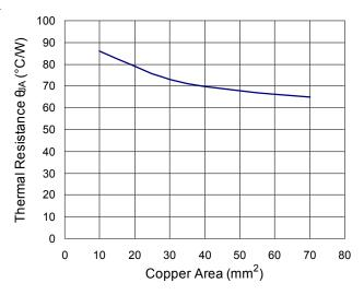
Figure 10. Relation Between Thermal Resistance  $\theta_{JA}$  and Copper Area
