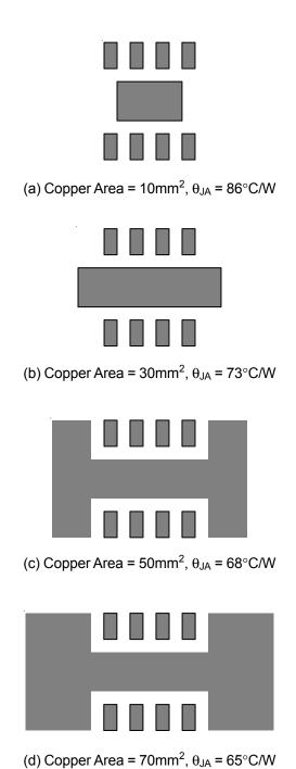
Figure 12. Thermal Resistance vs. Copper Area Layout Thermal Design
