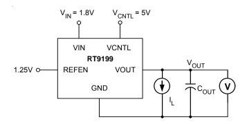
Figure 1. Output Voltage Tolerance, ΔV<sub>LOAD</sub>
