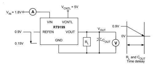
Figure 2. Current in Shutdown Mode, ISTBY
