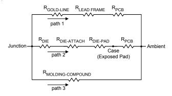
Figure 9. Thermal Resistance Equivalent Circuit
