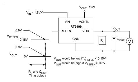
Figure 5. REFEN Pin Shutdown Threshold, VIH & VIL
