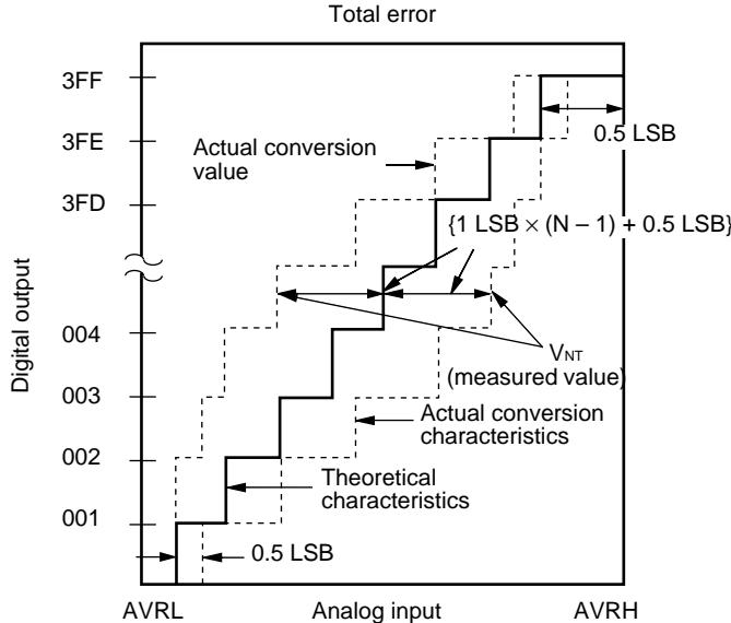
$$1 \text{ LSB} = (\text{Theoretical value}) \frac{\text{AVRH} - \text{AVRL}}{1024} [\text{V}]$$
