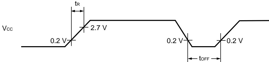
Sudden changes in the power supply voltage may cause a power-on reset.
