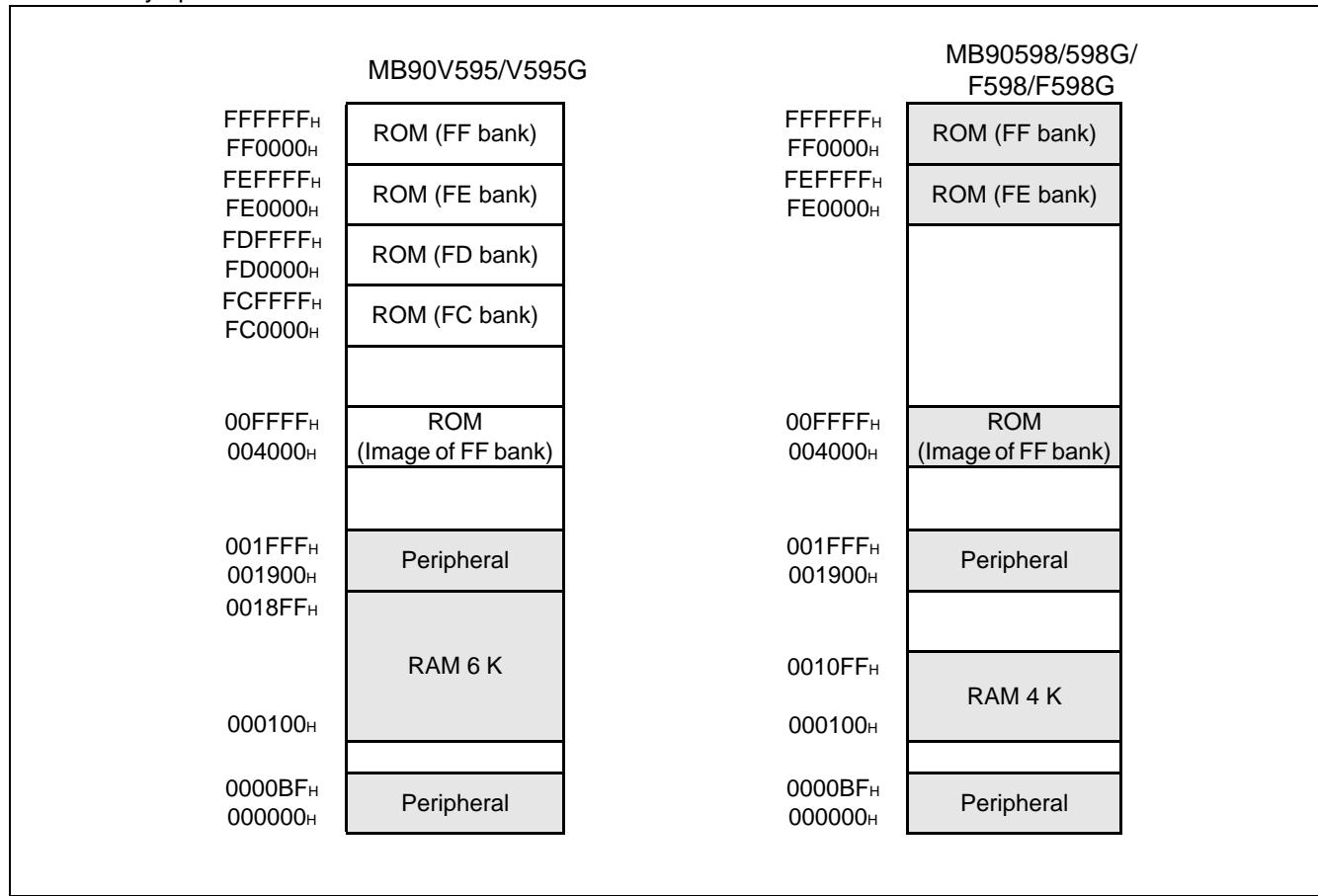
Note: The ROM data of bank FF is reflected in the upper address of bank 00, realizing effective use of the C compiler small model. The lower 16-bit of bank FF and the lower 16-bit of bank 00 are assigned to the same address, enabling reference of the table on the ROM without stating “far”.
