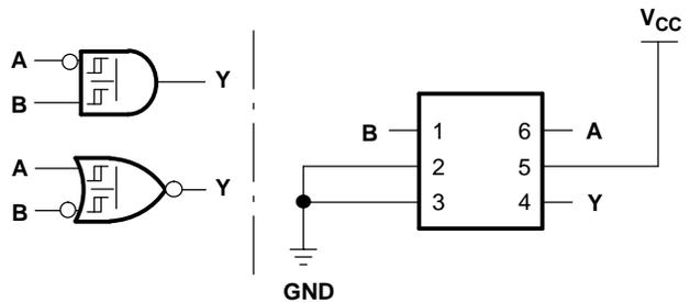
Figure 4. 2-Input AND Gate With One Inverted Input
