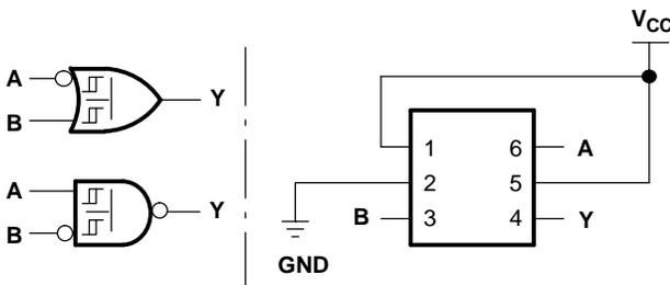
Figure 3. 2-Input OR Gate With One Inverted Input
