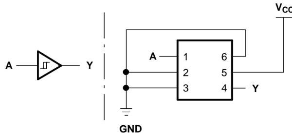
Figure 7. Noninverted Buffer
