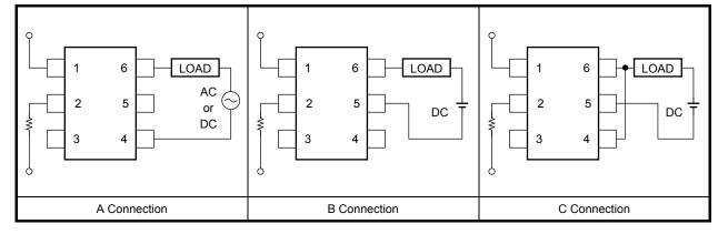
Note 1: Device considered a two-terminal device: LED side pins shorted together, and DETECTOR side pins shorted together.
