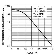
Figure 13. Voltage Gain as a Function of RADJ (Figure 2)
