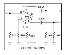
Figure 12. Voltage Gain Adjust Circuit
