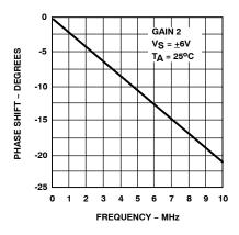
Figure 20. Phase Shift as a Function of Frequency
