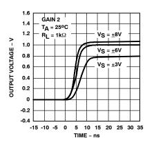
Figure 6. Pulse Response as a Function of Supply Voltage
