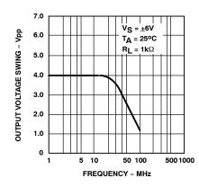
Figure 3. Output Voltage Swing as a Function of Frequency
