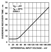
Figure 15. Differential Overdrive Recovery Time
