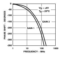
Figure 21. Phase Shift as a Function of Frequency
