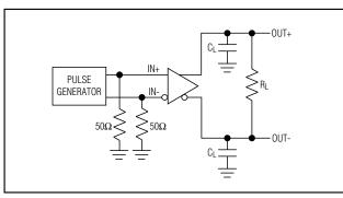
Figure 3. Transition Time and Propagation Delay Test Circuit
