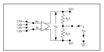
Figure 2. DC Load Test Circuit
