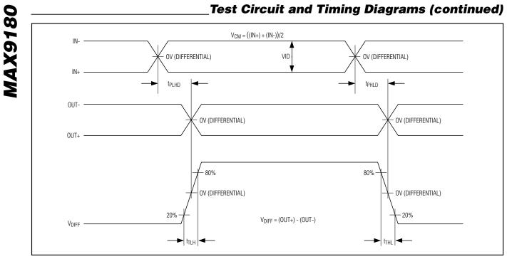
Figure 4. Transition Time and Propagation Delay Timing Diagram
