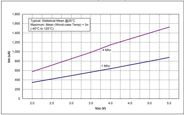
FIGURE 20-8: MAXIMUM IDD vs. VDD (EXTRC MODE)
