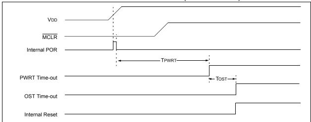
FIGURE 16-5: TIME-OUT SEQUENCE ON POWER-UP (DELAYED MCLR): CASE 2
