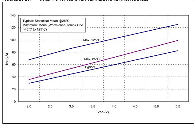
FIGURE 20-22: CVREF IPD vs. VDD OVER TEMPERATURE (LOW RANGE)
