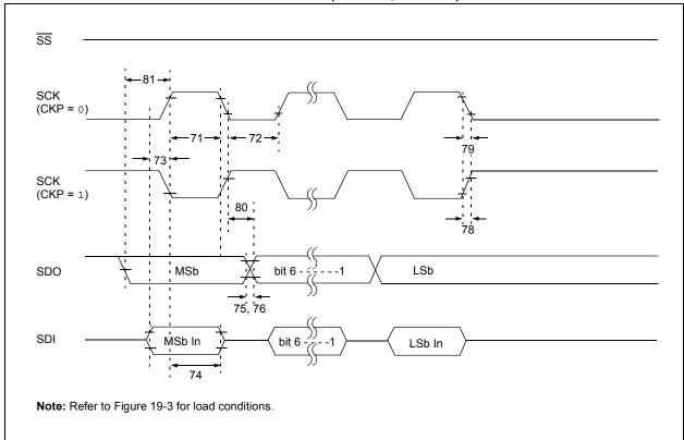
FIGURE 19-16: SPI SLAVE MODE TIMING (CKE = 0)
