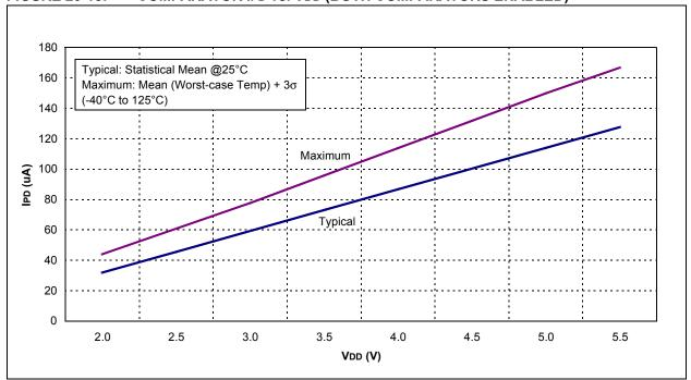
FIGURE 20-16: BOR IPD vs. VDD OVER TEMPERATURE
