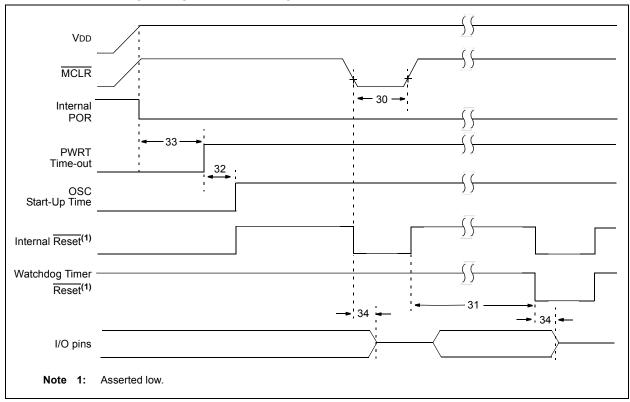
FIGURE 19-7: BROWN-OUT RESET TIMING AND CHARACTERISTICS
