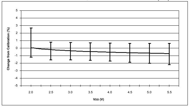
FIGURE 20-40: TYPICAL HFINTOSC FREQUENCY CHANGE vs. VDD (125°C)
