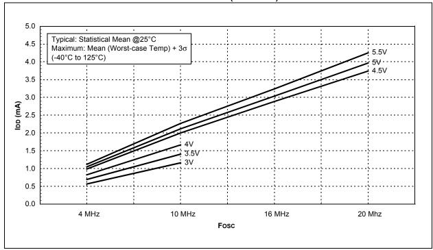
FIGURE 20-4: MAXIMUM IDD vs. FOSC OVER VDD (HS MODE)
