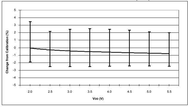
FIGURE 20-41: TYPICAL HFINTOSC FREQUENCY CHANGE vs. VDD (-40°C)
