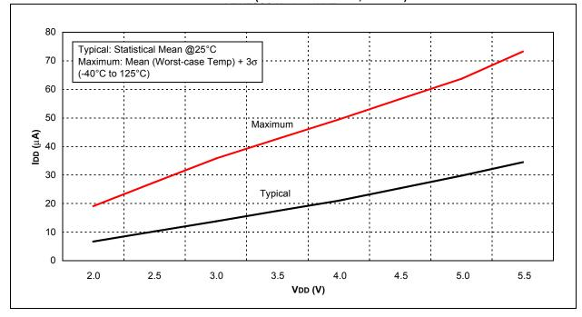
FIGURE 20-10: IDD vs. VDD (LP MODE)
