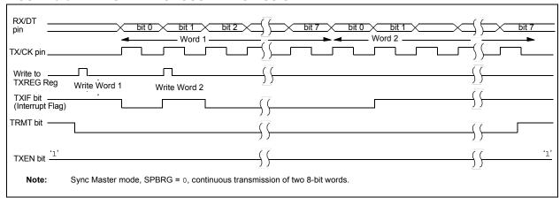
FIGURE 9-7: SYNCHRONOUS TRANSMISSION (THROUGH TXEN)
