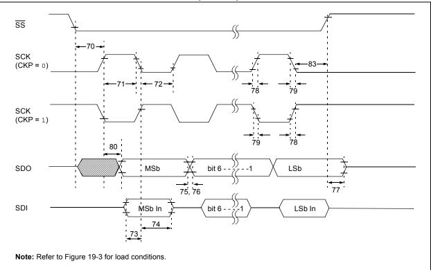
FIGURE 19-17: SPI SLAVE MODE TIMING (CKE = 1)
