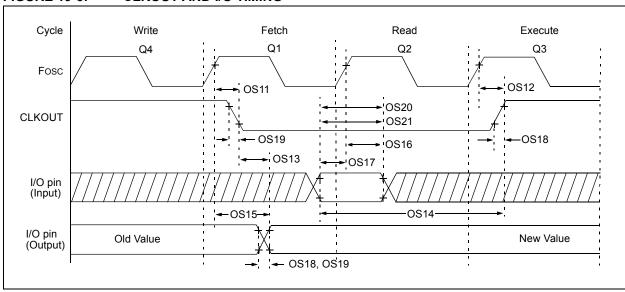
TABLE 19-3: CLKOUT AND I/O TIMING PARAMETERS
