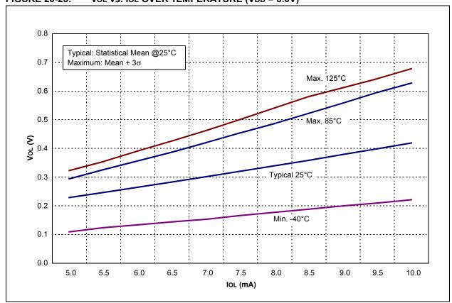
FIGURE 20-26: Vol vs. Iol OVER TEMPERATURE (VDD = 5.0V)
