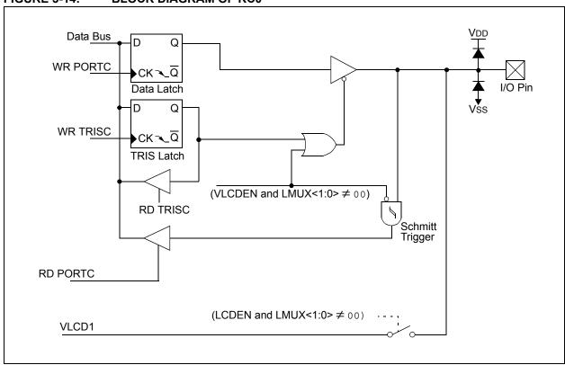
FIGURE 3-15: BLOCK DIAGRAM OF RC1
