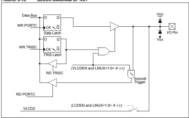
FIGURE 3-16: BLOCK DIAGRAM OF RC2
