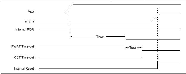
FIGURE 16-6: TIME-OUT SEQUENCE ON POWER-UP (MCLR WITH VDD): CASE 3
