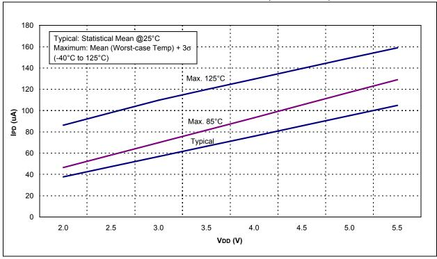
FIGURE 20-23: LVD IPD vs. VDD OVER TEMPERATURE
