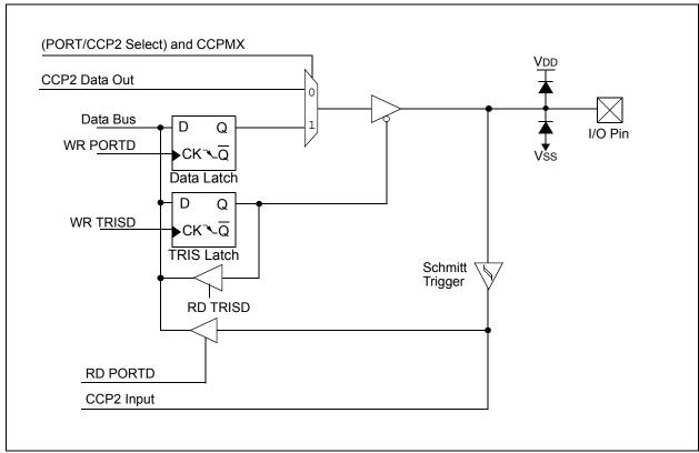
FIGURE 3-25: BLOCK DIAGRAM OF RD<7:3>
