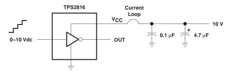
Figure 3. Shoot-Through Current Test Setup
