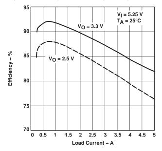
Figure 26. Converter Efficiency
