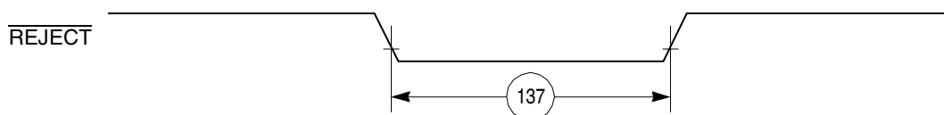
Figure 65. CAM Interface \overline{\text{REJECT}} Timing Diagram
