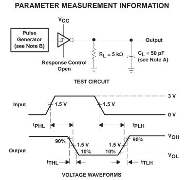
NOTES: A. C<sub>L</sub> includes probe and jig capacitances.
