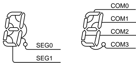
Figure 15-6 Example of COM, SEG Pin Connection (1/4 Duty)
