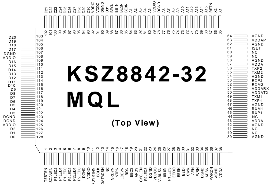
Figure 4. Standard – KSZ8842-32 MQL 128-Pin PQFP (Top View)
