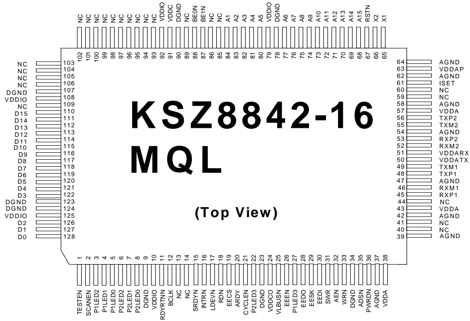
Figure 2. Standard – KSZ8842-16 MQL 128-Pin PQFP (Top View)
