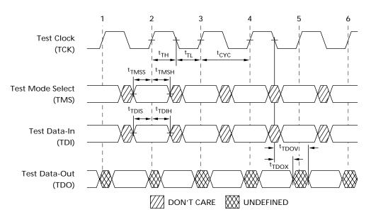
TAP AC Switching Characteristics Over the operating Range<sup>[9, 10]</sup>
