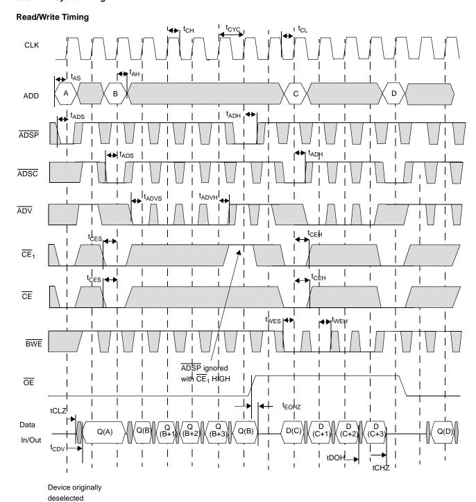
$\overline{\text{WE}}$  is the combination of  $\overline{\text{BWE}}$ ,  $\overline{\text{BW}}$ x, and  $\overline{\text{GW}}$  to define a Write cycle (see Write cycle description table).  $\overline{\text{CE}}$  is the combination of  $\overline{\text{CE}}_2$  and  $\overline{\text{CE}}_3$ . All chip selects need to be active in order to select the device. RAx stands for Read Address X, WAx stands for Write Address X, Dx stands for Data-in X, Qx stands for Data-out X.
