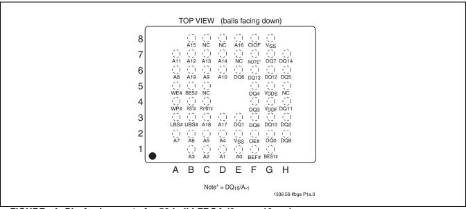
FIGURE 4: Pin Assignments for 56-ball LFBGA (8mm x 10mm)
