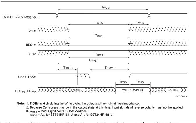
FIGURE 8: PSRAM Write Cycle Timing Diagram (UBS#, LBS# Controlled)<sup>1</sup> x16 PSRAM ONLY
