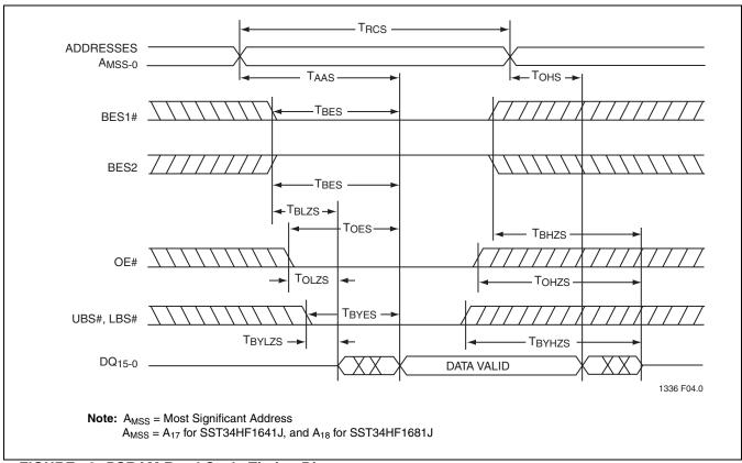
FIGURE 6: PSRAM Read Cycle Timing Diagram
