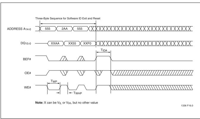
FIGURE 19: Flash Software ID Exit/CEI Exit for Word Mode (For Byte Mode A<sub>-1</sub> = 0)
