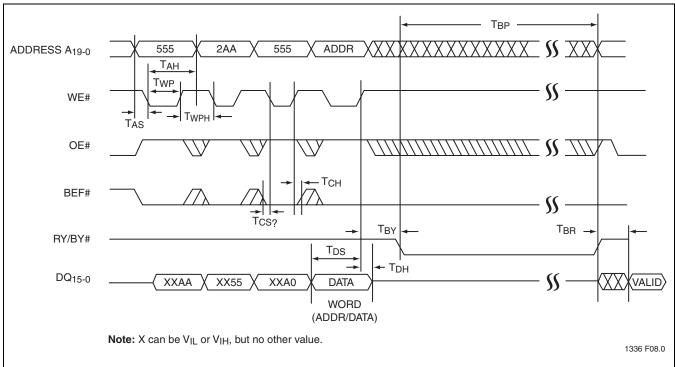
FIGURE 10: Flash WE# Controlled Program Cycle Timing Diagram for Word Mode (For Byte Mode A<sub>-1</sub> = Address Input)
