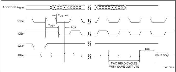
FIGURE 13: Flash Toggle Bit Timing Diagram for Word Mode (For Byte Mode A<sub>-1</sub> = Don't Care)
