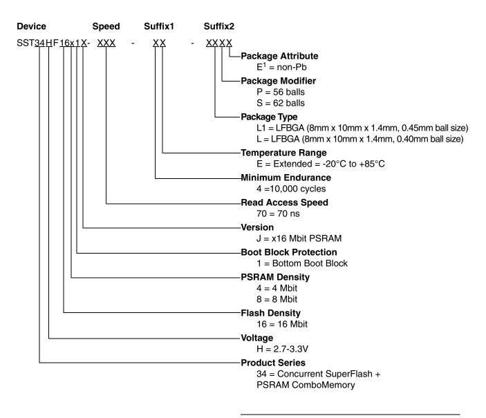
Environmental suffix "E" denotes non-Pb solder. SST non-Pb solder devices are "RoHS Compliant".
