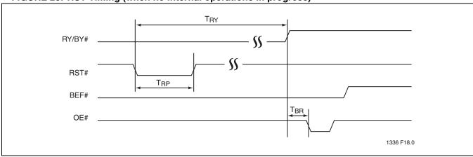
FIGURE 21: RST# Timing (during Sector- or Block-Erase operation)
