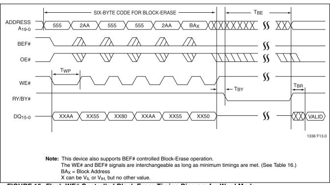
FIGURE 15: Flash WE# Controlled Block-Erase Timing Diagram for Word Mode (For Byte Mode A<sub>-1</sub> = Don't Care)
