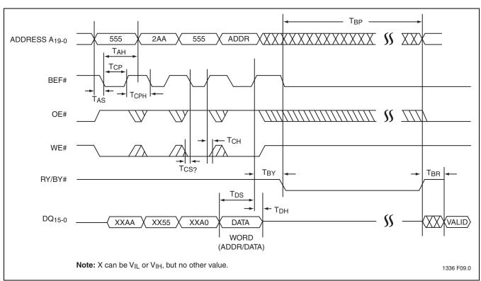
FIGURE 11: Flash BEF# Controlled Program Cycle Timing Diagram for Word Mode (For Byte Mode A<sub>-1</sub> = Address Input)
