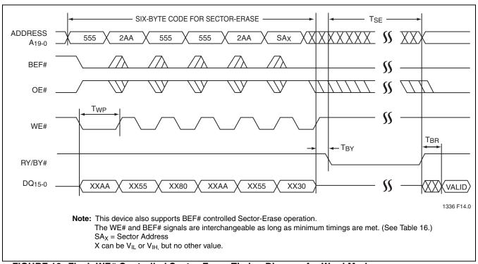
FIGURE 16: Flash WE# Controlled Sector-Erase Timing Diagram for Word Mode (For Byte Mode A<sub>-1</sub> = Don't Care)
