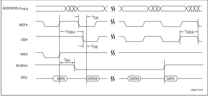
FIGURE 12: Flash Data# Polling Timing Diagram for Word Mode (For Byte Mode A<sub>-1</sub> = Address Input)
