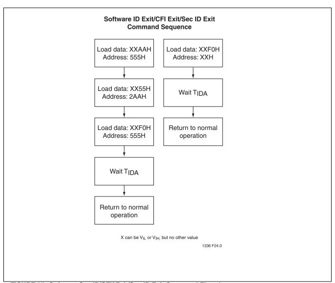
FIGURE 27: Software Sec ID/CFI/ Exit/Sec ID Exit Command Flowcharts
