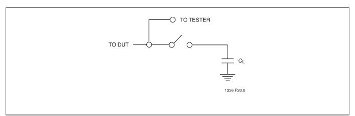
FIGURE 23: A Test Load Example
