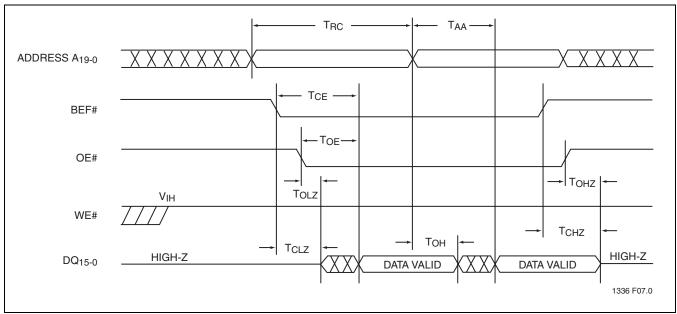
FIGURE 9: Flash Read Cycle Timing Diagram for Word Mode (For Byte Mode A<sub>-1</sub> = Address Input)
