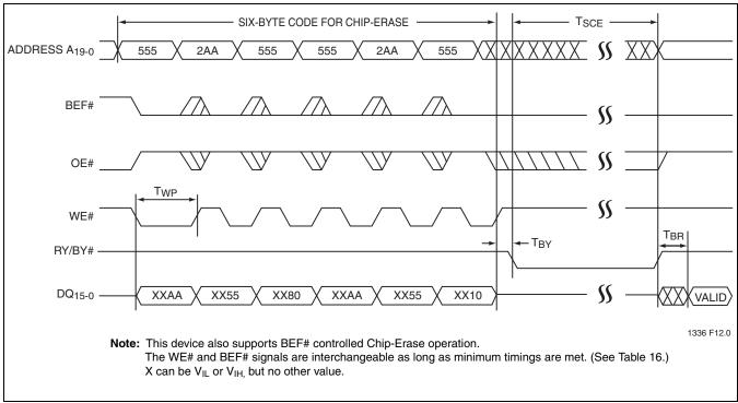
FIGURE 14: Flash WE# Controlled Chip-Erase Timing Diagram for Word Mode (For Byte Mode A<sub>-1</sub> = Don't Care)
