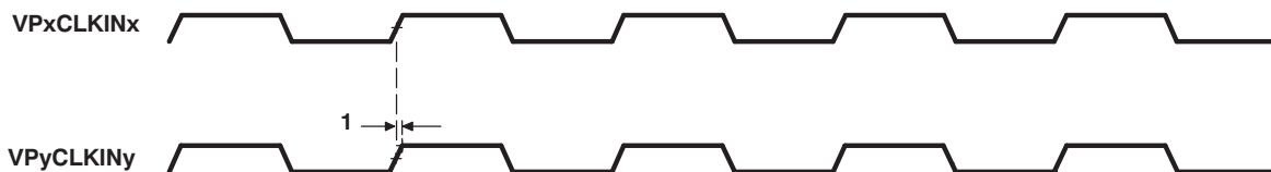
Figure 6-25. Video Port Dual-Display Sync Timing
