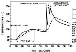
BOTTOM SIDE OF PC BOARD CONVEYOR SPEED = 1.83 M/MIN (6 FT/MIN) PREHEAT SETTING = 150°C (100°C PCB) SOLDER WAVE TEMPERATURE = 245°C AIR KNIFE AIR TEMPERATURE = 390°C AIR KNIFE DISTANCE = 1.91 mm (0.25 IN.) AIR KNIFE ANGLE = 40° SOLDER: SN63; FLUX: RMA NOTE: ALLOW FOR BOARDS TO BE SUFFICIENTLY COOLED BEFORE EXERTING MECHANICAL FORCE.
