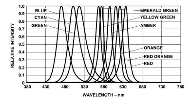
Figure 1. Relative Intensity Vs. Wavelength.
