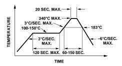
Figure 9a. Recommended SnPb Reflow Soldering Profile.
