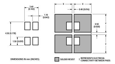
Figure 8a. Recommended Soldering Pad Pattern.
