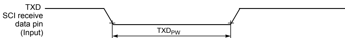
Figure 4-32 TXD Pulse Width
