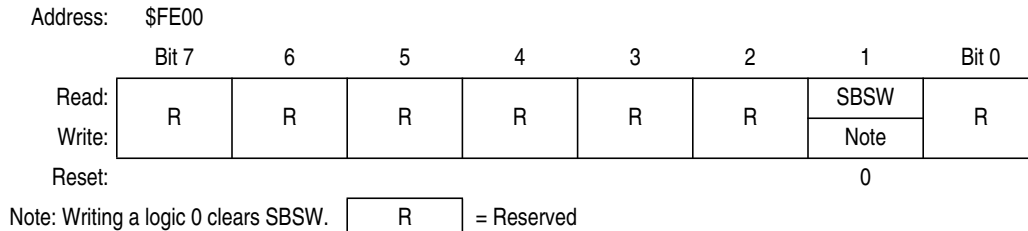
Figure 7-20. SIM Break Status Register (SBSR)
