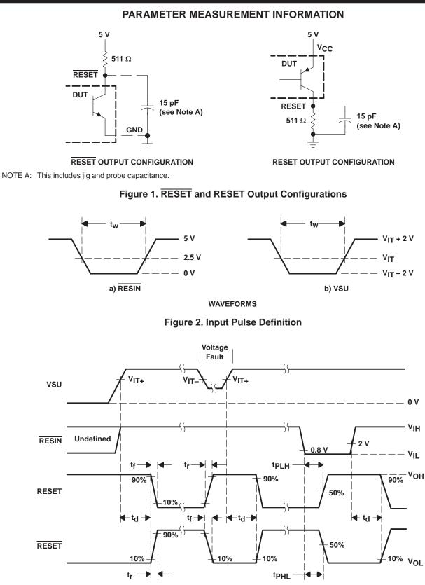
Figure 3. Voltage Waveforms
