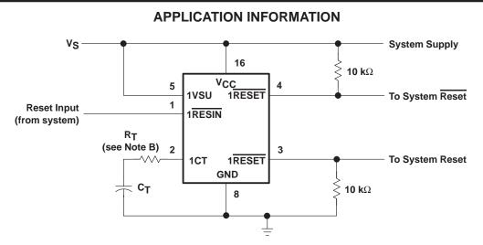
NOTE B: When V<sub>CC</sub> and 1VSU are connected to the same point, it is recommended that series resistance (R<sub>T</sub>) be added between the time-delay programming capacitor (C<sub>T</sub>) and the voltage-supervisor device terminal (1CT). The suggested R<sub>T</sub> value is given by:
