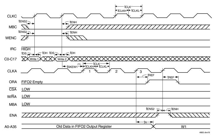
Figure 18. ORA Flag Timing and First Data Word Fall through when FIFO2 is Empty (FWFT Mode)
