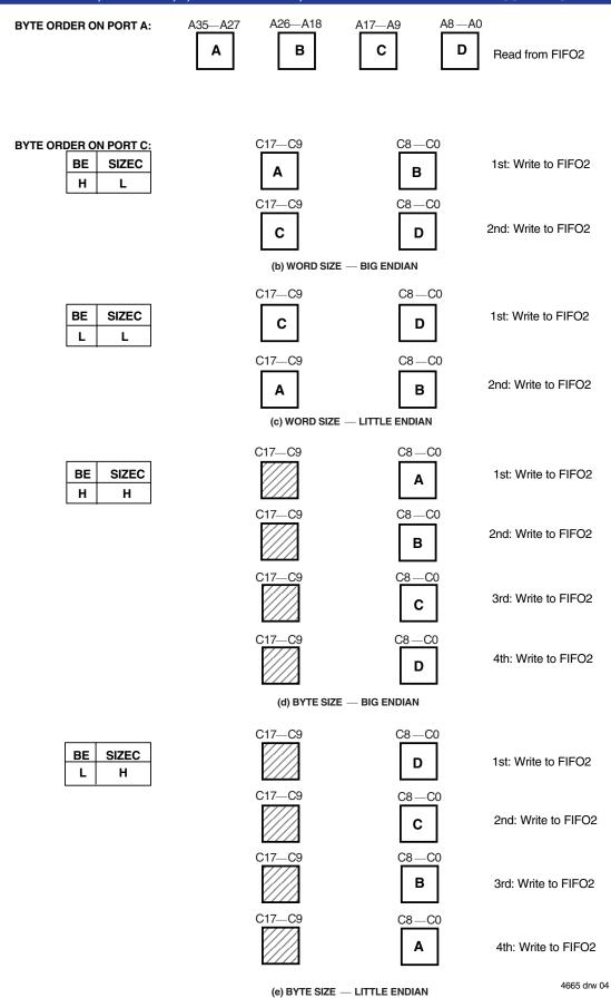
Figure 3. Port C Bus Sizing
