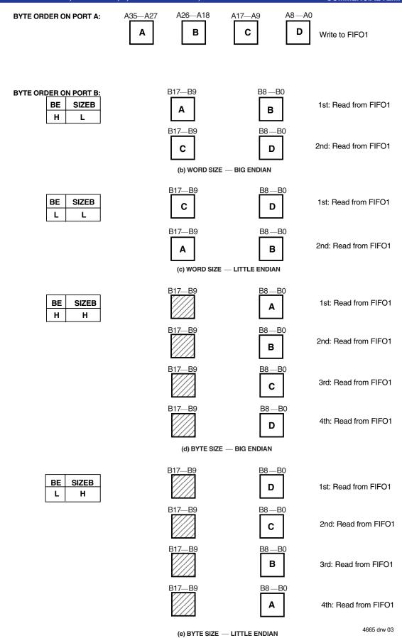
Figure 2. Port B Bus Sizing
