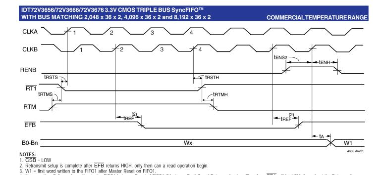
Figure 30. Retransmit Timing for FIFO1 (IDT Standard Mode)
