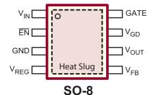
Backside on the SO-8 package is at ground potential and may be connected to ground or left unconnected.
