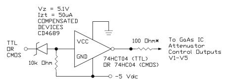
Simple driver using inexpensive standard logic ICs provides fast switching using minimum DC current. \* Recommended value to suppress unwanted RF signals at V1 - V5 control lines.
