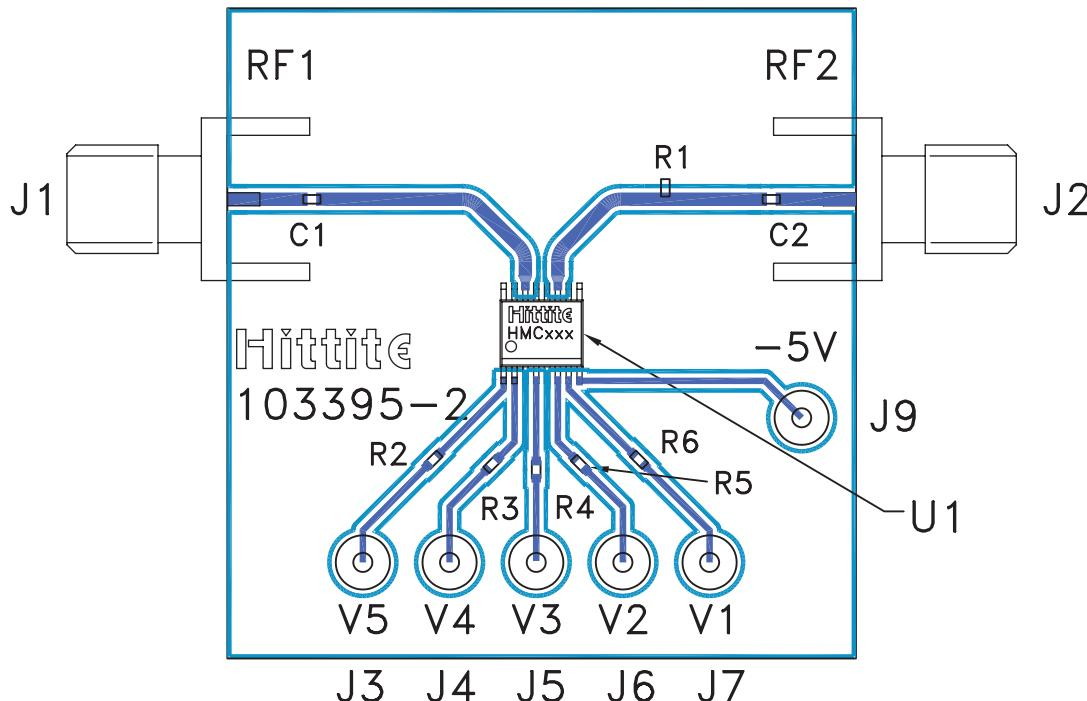
\*  $R_2 - R_6 = 100\text{ Ohm}$ .
