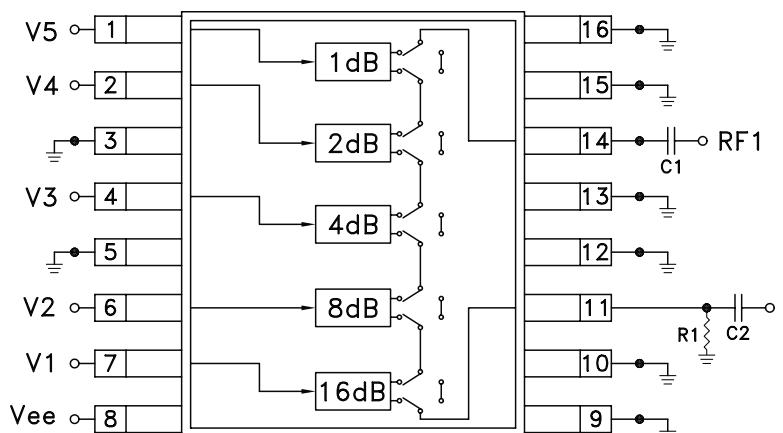
DC Blocking Capacitors C1 & C2 are required on RF1 & RF2. Choose C1 = C2 = 100 pF ~ 0.1 uF to allow lowest customer specific frequency to pass with minimal loss. R1= 5K Ohm is required to supply voltage to the circuit through either Pin 11 or Pin 14.
