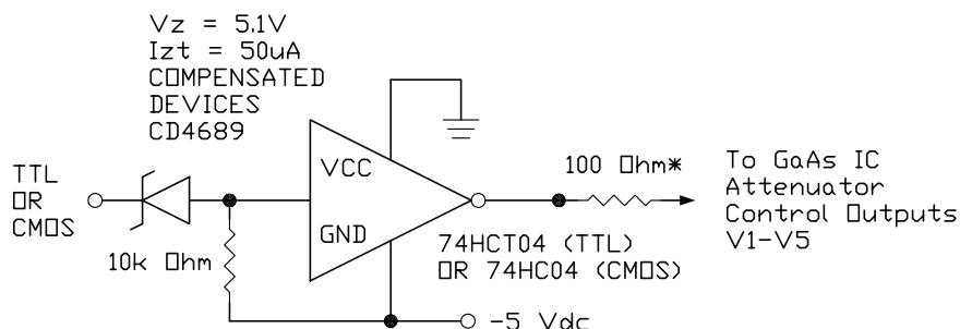
Simple driver using inexpensive standard logic ICs provides fast switching using minimum DC current. \* Recommended value to suppress unwanted RF signals at V1 - V5 control lines.
