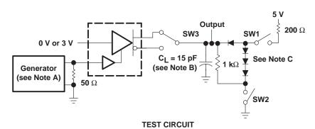
Output Output 3 V **Enable Input Enable Input** 1.5 V SW1 Closed V<sub>OH</sub> SW1 Closed SW2 Open SW2 Closed Output Output Vol tPZH tpLZ → ۷он SW1 Closed Output Output SW1 Open SW2 Closed SW2 Closed
