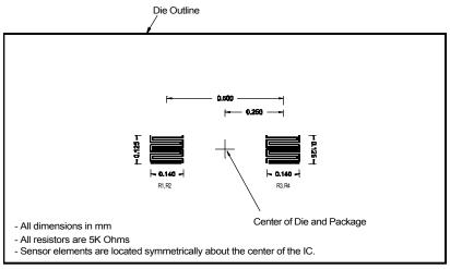
Note: ABL006 Sensor Element Size and Spacing Not Shown
