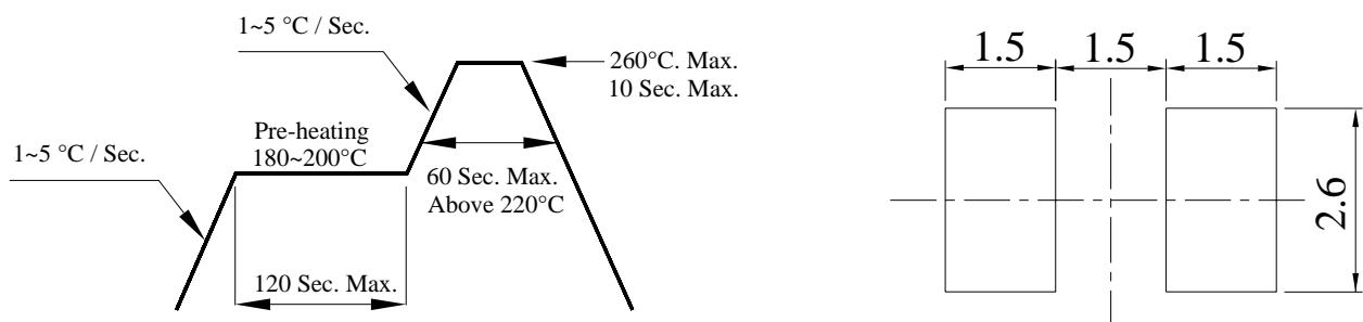
3.2 Reflow soldering should not be done more than two times.
