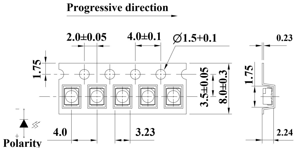
**Note:** The tolerances unless mentioned is  $\pm 0.1\text{mm}$
