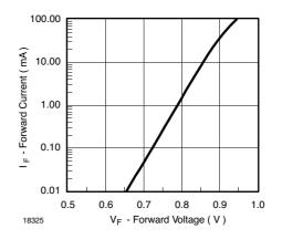
Fig. 3 Forward Current vs. Forward Voltage
