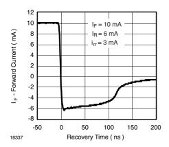
Fig. 5 Typical Charge Recovery Curve
