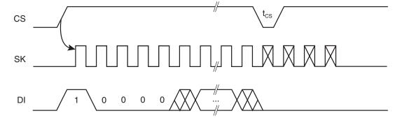
Figure 6. WRITE Timing
