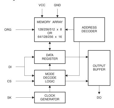
Note: When the ORG pin is connected to VCC, the "x 16" organization is selected. When it is connected to ground, the "x 8" organization is selected. If the ORG pin is left unconnected and the application does not load the input beyond the capability of the internal 1 Meg ohm pullup, then the "x 16" organization is selected. The feature is not available on the 1.8V devices.
