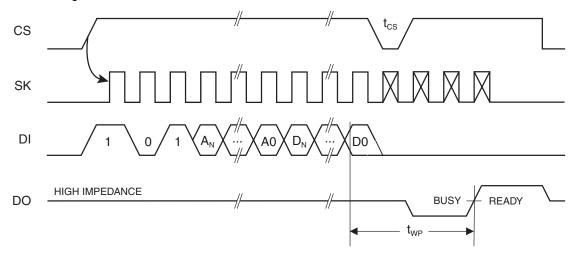
Figure 7. WRAL Timing<sup>(1)</sup>
