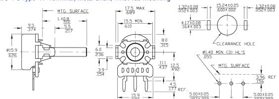
T057-C2-270 Solder Lug Terminal SPST Switch, Solder Lug Terminals, Concentric Metal Shafts, Bushing Mount
