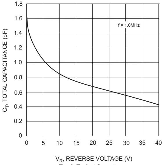
Fig. 3 Typical Capacitance
