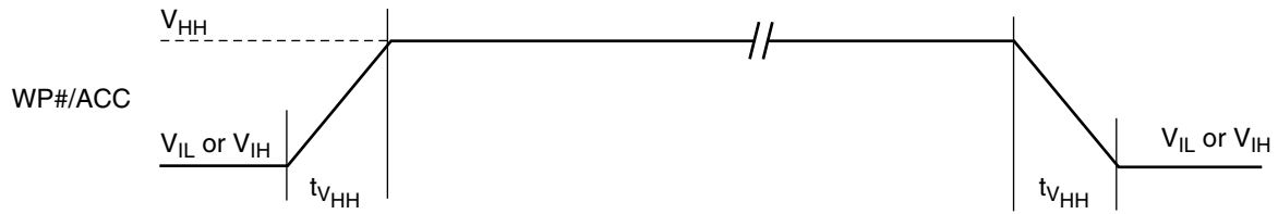
Figure 23. Accelerated Program Timing Diagram
