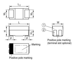
① Encapsulation: molded epoxy resin
