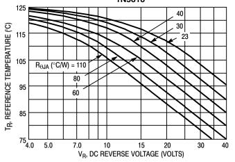
Figure 3. Maximum Reference Temperature
