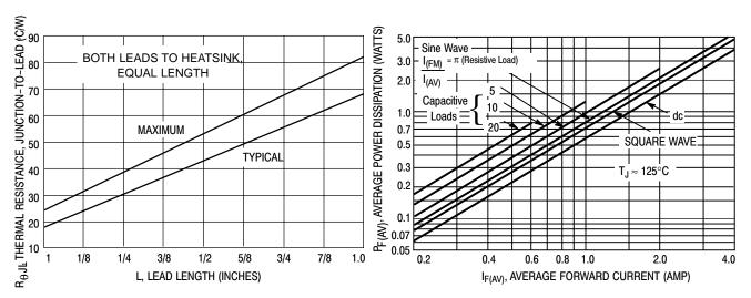
Figure 4. Steady-State Thermal Resistance
