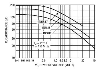
Figure 10. Typical Capacitance
