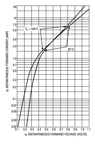
Figure 7. Typical Forward Voltage
