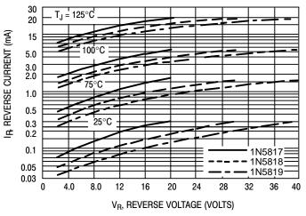
**Figure 9. Typical Reverse Current**
