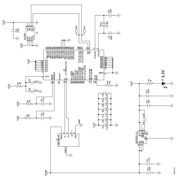
Figure 36. EVAL-ADG2188EB Schematic, USB Controller Section
