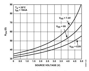
Figure 7.  $R_{ON}$  vs. Source Voltage,  $V_{DD}$  = 8 V  $\pm$  10%
