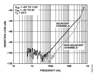
Figure 21. Crosstalk vs. Frequency
