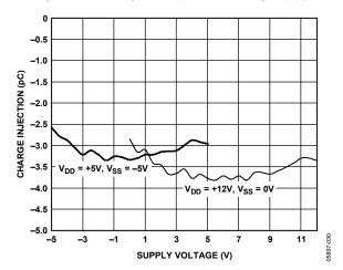
Figure 15. Charge Injection vs. Supply Voltage
