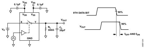
Figure 28. Switching Times, ton, toff
