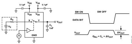
Figure 29. Charge Injection
