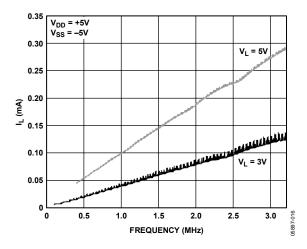
Figure 22. Digital Current (I<sub>L</sub>) vs. Frequency
