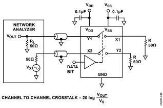
Figure 32. Channel-to-Channel Crosstalk
