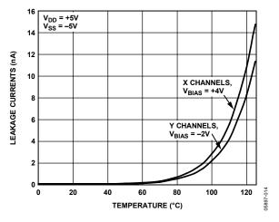
Figure 11. On Leakage vs. Temperature, Dual ±5 V Supplies
