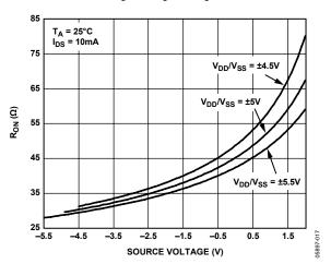
Figure 5. R<sub>ON</sub> vs. Source Voltage, Dual ±5 V Supplies
