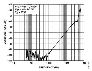
Figure 20. Off Isolation vs. Frequency
