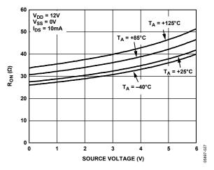
Figure 9.  $R_{ON}$  vs. Temperature,  $V_{DD} = 12 V$
