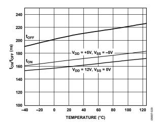
Figure 16. t<sub>ON</sub>/t<sub>OFF</sub> Times vs. Temperature
