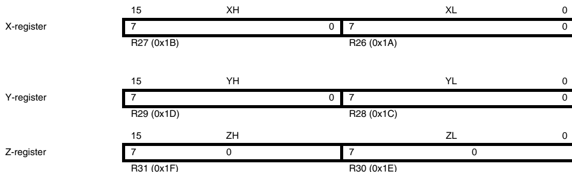
Figure 5-3. The X-, Y-, and Z-registers
