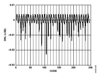
Figure 60. AD9704 Typical Uncalibrated DNL
