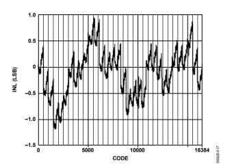
Figure 19. Typical Uncalibrated INL
