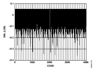
Figure 64. AD9706 Typical Uncalibrated DNL
