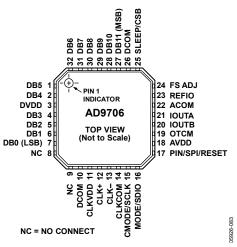
Figure 4. AD9706 Pin Configuration
