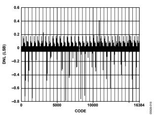
Figure 20. Typical Uncalibrated DNL
