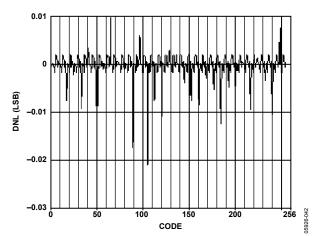
Figure 47. AD9704 Typical Uncalibrated DNL
