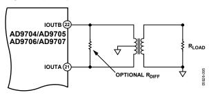
Figure 90. Differential Output Using a Transformer
