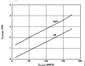
Figure 86. ICLKVDD vs. fcLOCK @ CLKVDD = 3.3 V
