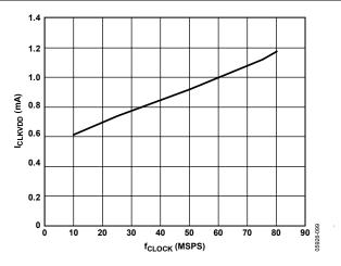
Figure 87. I<sub>CLKVDD</sub> vs. f<sub>CLOCK</sub> (Differential Clock Mode) @ CLKVDD = 1.8 V
