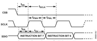
Figure 77. Timing Diagram for SPI Register Write
