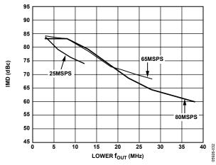
Figure 36. Dual-Tone IMD vs.  $f_{OUT} @ I_{OUTFS} = 2 \text{ mA}$  and 0 dBFS
