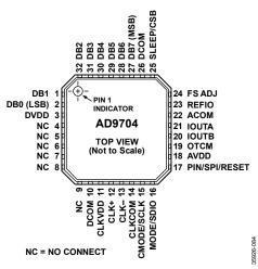
Figure 6. AD9704 Pin Configuration
