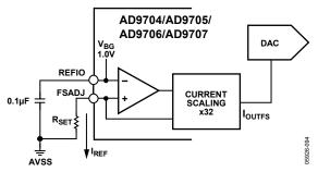
Figure 79. Internal Reference Configuration
