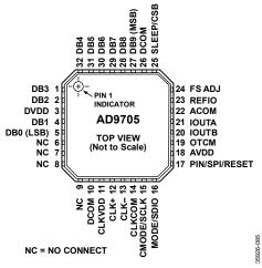
Figure 5. AD9705 Pin Configuration
