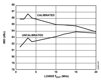
Figure 89. IMD vs.  $f_{OUT}$  @ 175 MSPS and  $I_{OUTFS} = 2 \text{ mA}$
