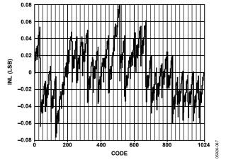
Figure 61. AD9705 Typical Uncalibrated INL
