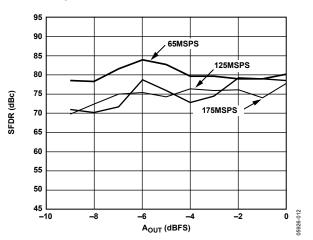
Figure 14. Single-Tone SFDR vs.  $A_{OUT} @ f_{OUT} = f_{CLOCK}/5$
