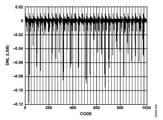
Figure 62. AD9705 Typical Uncalibrated DNL
