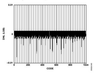
Figure 49. AD9705 Typical Uncalibrated DNL
