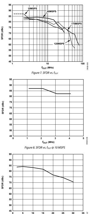
$f_{OUT}$  (MHz) Figure 9. SFDR vs. f<sub>OUT</sub> @ 65 MSPS
