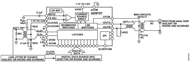
Figure 71. Basic AC Characterization Test Setup
