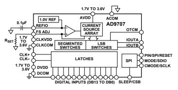
Figure 72. Simplified Block Diagram
