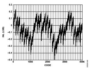
Figure 50. AD9706 Typical Uncalibrated INL
