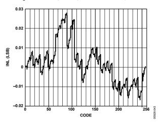
Figure 46. AD9704 Typical Uncalibrated INL
