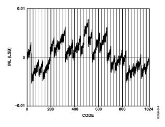
Figure 48. AD9705 Typical Uncalibrated INL
