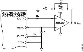
Figure 91. Single-Supply Single-Ended Buffer
