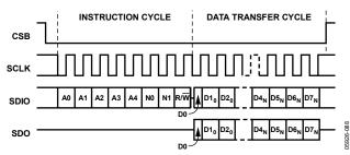
Figure 76. Serial Register Interface Timing, LSB First Read
