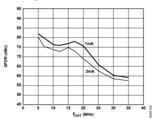
Figure 32. SFDR vs. f<sub>OUT</sub> and I<sub>OUTFS</sub> @ 80 MSPS
