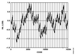
Figure 39. Typical Uncalibrated INL
