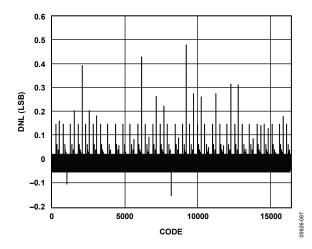
Figure 22. Typical Calibrated DNL
