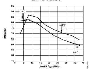
Figure 38. Dual-Tone IMD vs.  $f_{OUT}$  and Temperature @ 80 MSPS,  $I_{OUTFS} = 2 \text{ mA}$  and 0 dBFS
