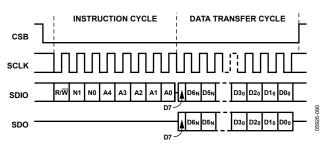
Figure 74. Serial Register Interface Timing, MSB First Read
