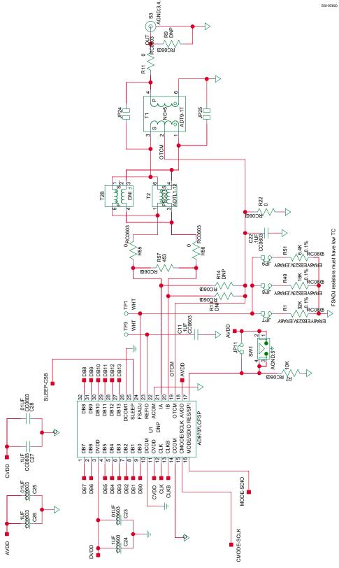
Figure 94. Output Signal Conditioning
