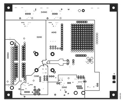
Figure 102. Layer 2—Ground Plane
