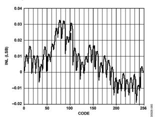
Figure 59. AD9704 Typical Uncalibrated INL
