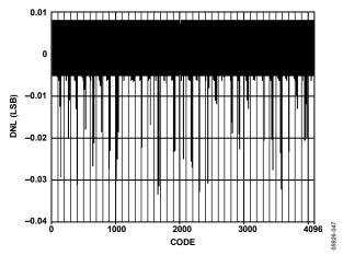
Figure 51. AD9706 Typical Uncalibrated DNL
