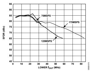
Figure 17. Dual-Tone IMD vs. f<sub>OUT</sub> @ 0 dBFS
