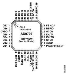
Figure 3. AD9707 Pin Configuration
