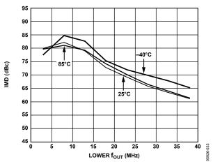
Figure 37. Dual-Tone IMD vs.  $f_{OUT}$  and Temperature @ 80 MSPS,  $I_{OUTFS} = 1 \text{ mA}$  and 0 dBFS
