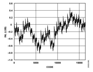
Figure 21. Typical Calibrated INL
