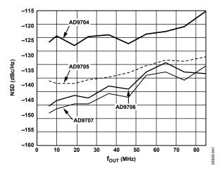
Figure 45. AD9704, AD9705, AD9706 NSD vs. fout @ 0 dBFS
