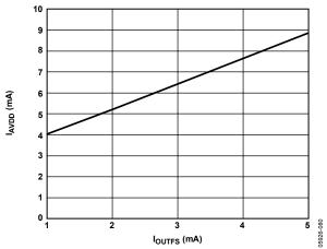
Figure 82.  $I_{AVDD}$  vs.  $I_{OUTFS}$  @ AVDD = 3.3 V
