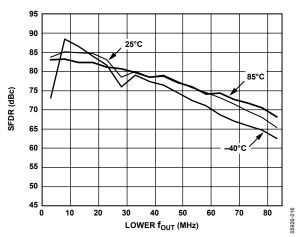
Figure 18. Dual-Tone IMD vs.  $f_{\text{OUT}}$  and Temperature @ 0 dBFS
