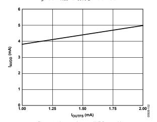
Figure 83.  $I_{AVDD}$  vs.  $I_{OUTFS}$  @ AVDD = 1.8 V
