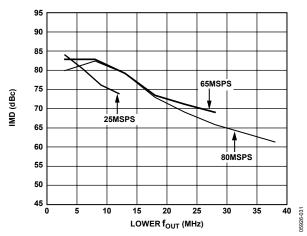
Figure 35. Dual-Tone IMD vs.  $f_{OUT} @ I_{OUTFS} = 1 \text{ mA}$  and 0 dBFS
