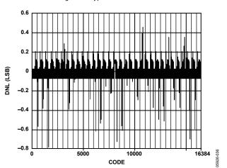
Figure 40. Typical Uncalibrated DNL
