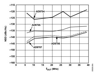
Figure 58. AD9704, AD9705, AD9706 NSD vs. fout @ 0 dBFS
