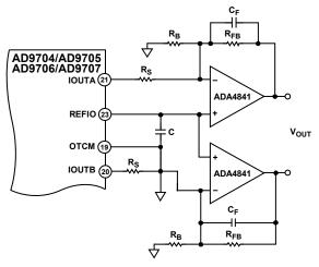
Figure 92. Single-Supply Differential Buffer
