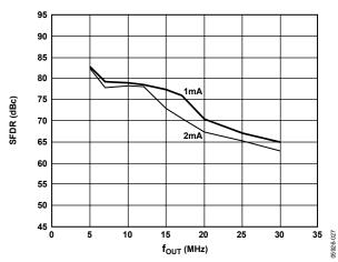
Figure 31. SFDR vs. f<sub>OUT</sub> and I<sub>OUTFS</sub> @ 65 MSPS
