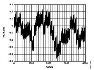
Figure 63. AD9706 Typical Uncalibrated INL
