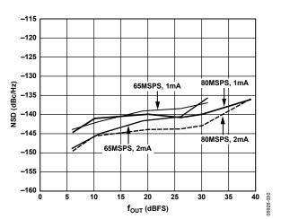
Figure 34. NSD vs.  $f_{\text{OUT}}$ ,  $f_{\text{CLOCK}}$ , and  $I_{\text{OUTFS}} @ 0 \text{ dBFS}$
