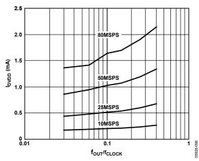
Figure 85. IDVDD vs. fout/fclock Ratio @ DVDD = 1.8 V
