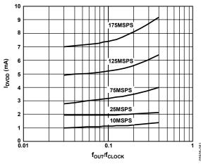
Figure 84.  $I_{DVDD}$  vs.  $f_{OUT}/f_{CLOCK}$  Ratio @ DVDD = 3.3 V
